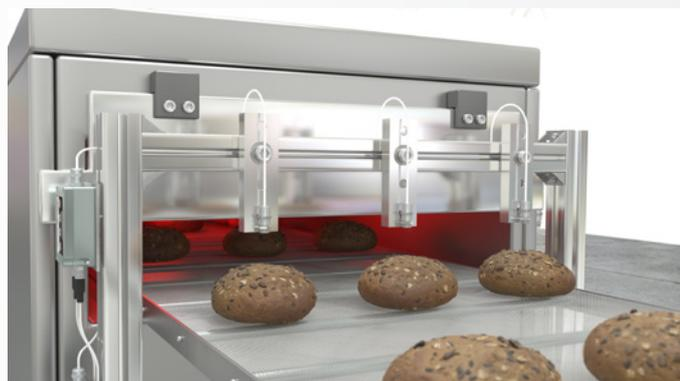
Measuring the temperature of baked goods with thermoMETER UC sensors
