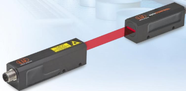
Light source and receiver can be mounted at any distance up to 5 m from each other. All models can be mounted both vertically and horizontally without additional brackets. The compact design of the housings and the 90° design allow the miniature micrometers to be mounted even in confined installation spaces. In addition the analog output, an adjustable limit switch is included. This can be operated in NPN (light switching) as well as in PNP logic (dark switching).
