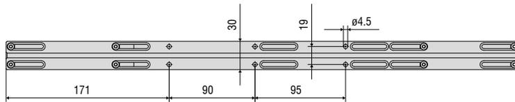
Light source and receiver with mounting rail
