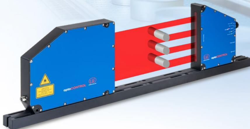
The optoCONTROL 2520-95 is a compact laser micrometer that features excellent linearity and high accuracy with a large measuring range of 95 mm. The optoCONTROL 2520-95 is flexible; the measuring object can be placed at any position within the light curtain and the distance from the light source to the receiver can be freely selected.
