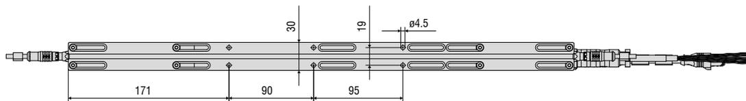
**Light source and receiver with mounting rail**
