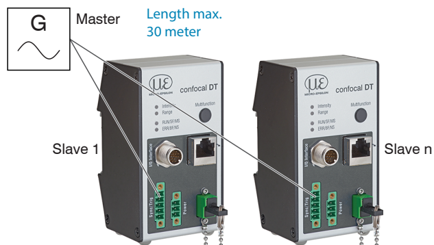
Fig. 4.16: Synchronization of multiple controllers, star-shaped
