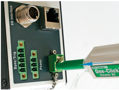
Fig. 17.4: One-Click™ Cleaner for cleaning E2000 optical fiber transitions
