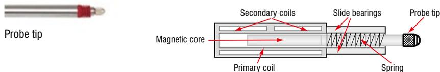
Measuring principle displacement sensor
