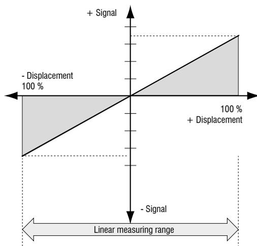
Measuring principle gauging sensor
