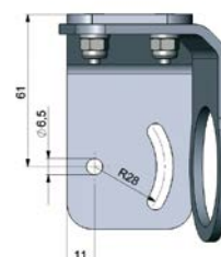
TM-AB-CTL Mounting bracket (adjustable)
